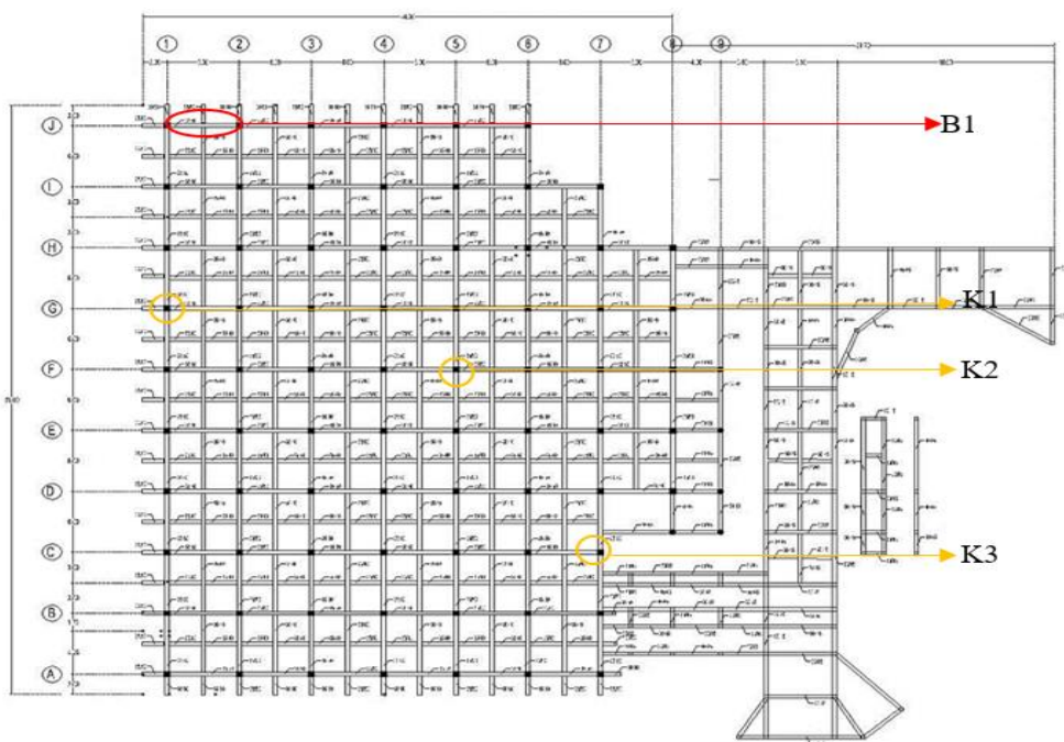
Figure 2. Plan for taking the uniformity of concrete quality in beams and columns on Floor 2 of the UMBCC building
