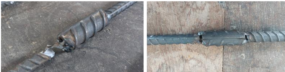
Figure 14. Failure of welded joints in D13 and D16 reinforcement splices
