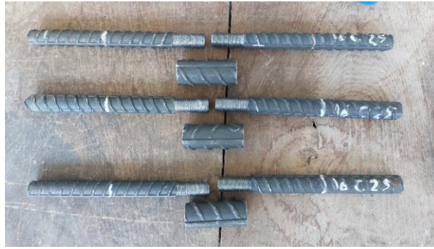
Figure 12. Failure did not reach fracture for D16
