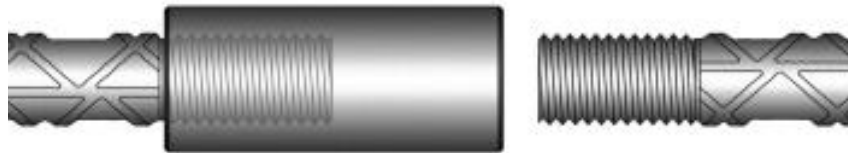
Figure 2. Threaded coupler with standard national coarse threads (ACI Committee 439, 2007)
