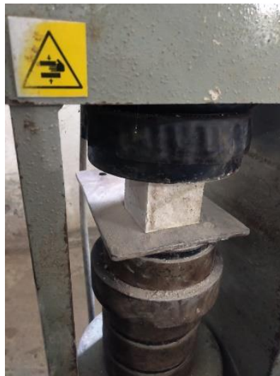
Figure 2. Concrete compression testing
