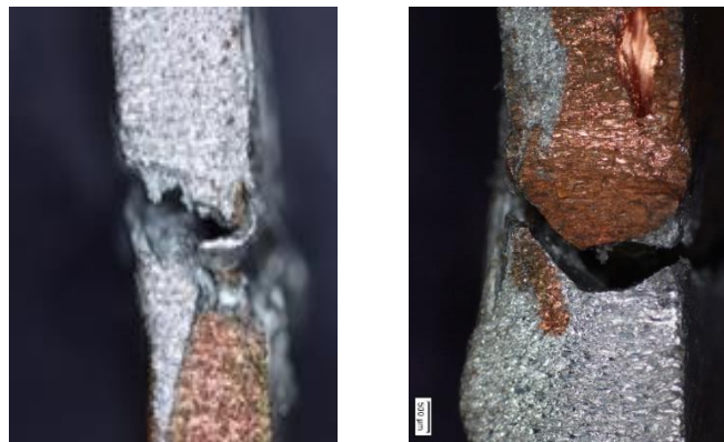
Figure 6. Fracture features of tensile specimens' friction stir welded at (a) 550 rpm, (b) 2280 rpm
