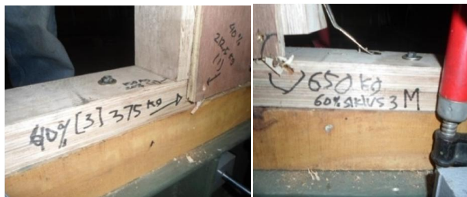
(b) Nail Pull-Through of Sheathing (d) Pull-Through Sheathing Failures
