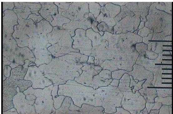
GAMBAR 6. Struktur mikro pada daerah HAZ (*Heat Affected Zone*)
