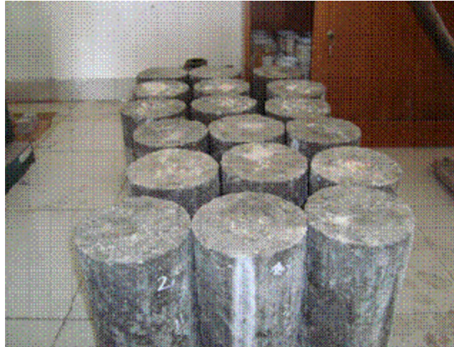
GAMBAR 3. Benda uji silinder beton-agregat bambu
