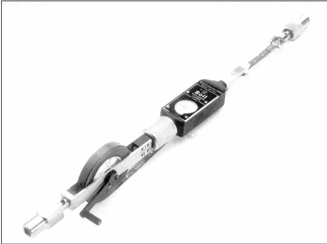
FIGURE 4. Tape extensometer used in dike 18 monitoring
